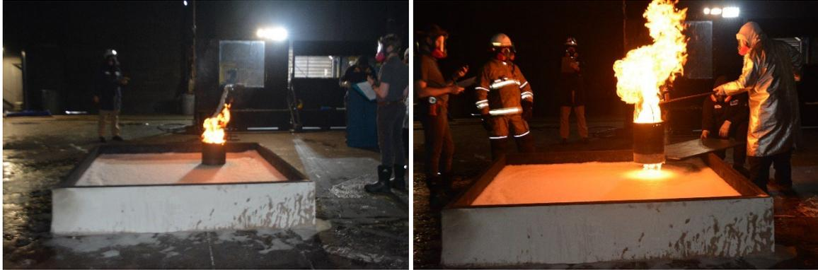
**Figure 10. Start of Burnback Test (Left) and Removal of Stovepipe (Right).**
