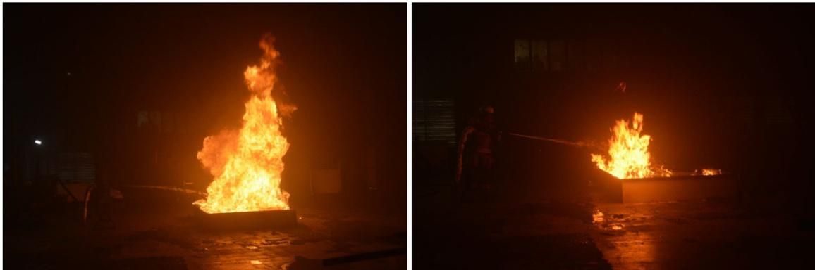
**Figure 7. Foam Discharge Prior to (Left) and After (Right) Control Time.**
