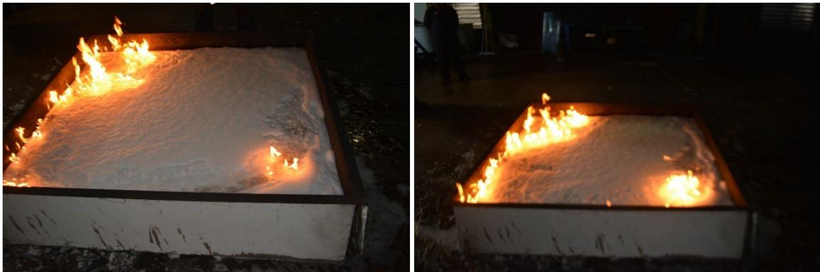
**Figure 12. Additional Flame Spread During Burnback Test.**
