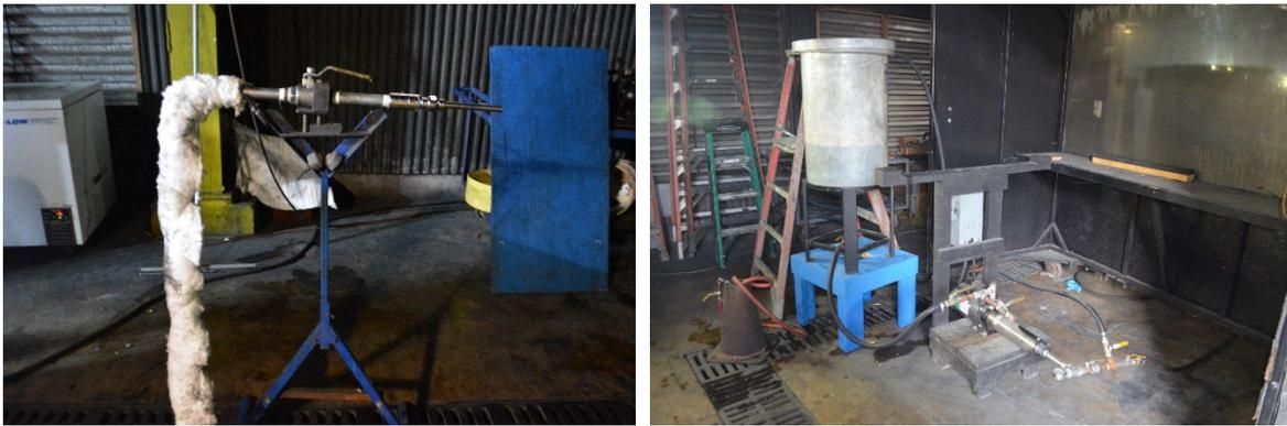
**Figure 5. Special Fire Test Equipment (Left: Discharge Nozzle, Right: SwRI Pump and Tank).**
